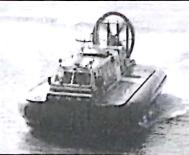
A hovercraft is supported on a cushion of air. Aside from travelling on water, it can also travel on different types of terrain such as soft mud, marshes, swamps as well as on firm ground. There is an increasing number of small hovercrafts used for fun and racing purposes, mainly on lakes, marshy areas and some estuaries.
